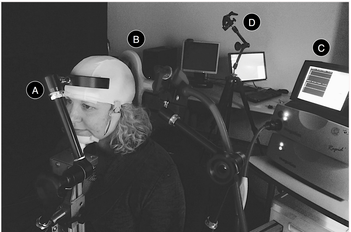
Fig 3. TMS Components of the BBI for the Inquirer. During the experiment, the inquirer sat in front of a computer screen on a BrainSight chair, with his or her head kept in place by a two-pronged head rest (A). A figure-of-8 TMS coil (B), connected to a MagStim Super Rapid 2 stimulator (C) was positioned over the inquirer's occipital lobe to deliver visual stimulation in accordance with the respondent's answer. The head position and the coil position were carefully checked with the aid of a laser pointer (D).
